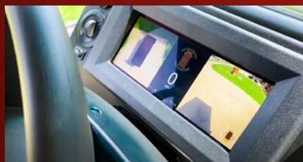
360° Camera System with Proximity Sensors
